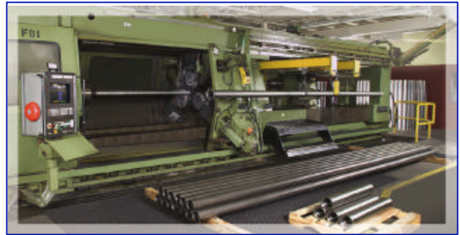
On the right of the photo is a pallet with four extruded Titanium preforms on it. In between the preforms and the flowforming machine is a stack of 24 foot long flowformed 4" schedule 10 pipe.
