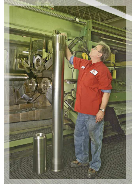
Nickel preform on the left with flowformed component on the right.
