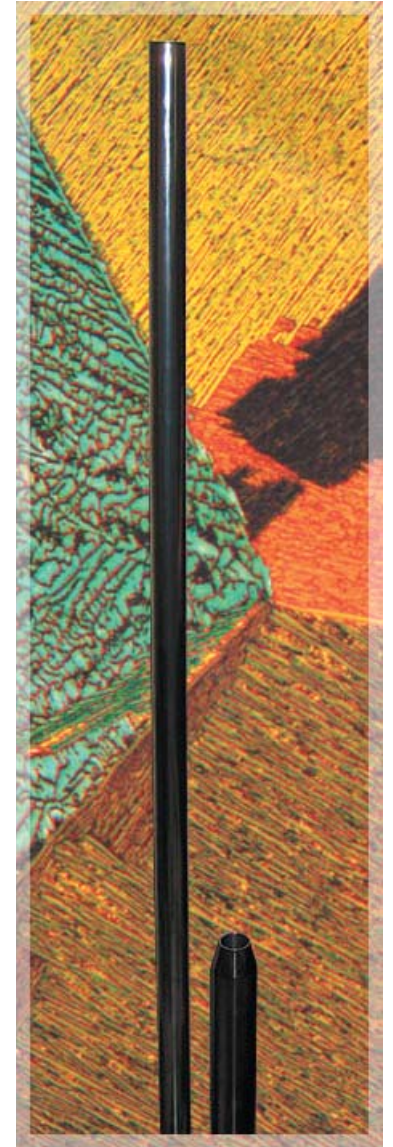
Flowformed Inconel 718 60" tube on the left and 15" preform on the right
