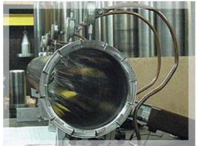
Flowformed Inconel 718 with 8 micro inch finish on the ID
